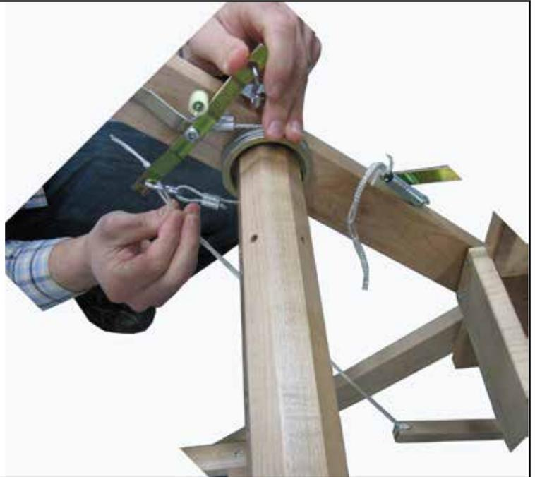
Join the front “S” hook of the brake lever to the brake spring
