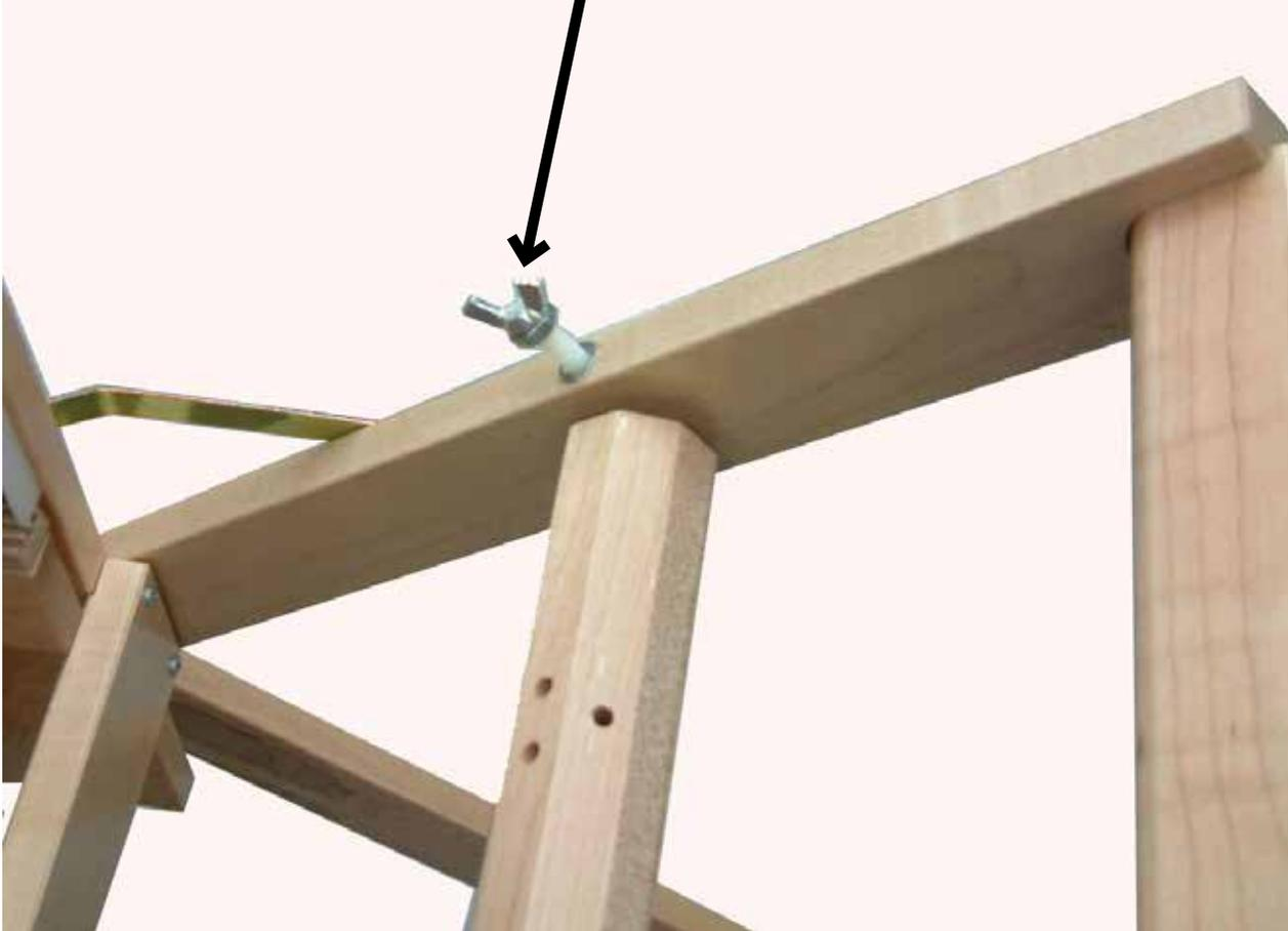
Install the Warp beam advance control system.
