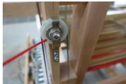
3- Spray into the ball bearing pulleys.
