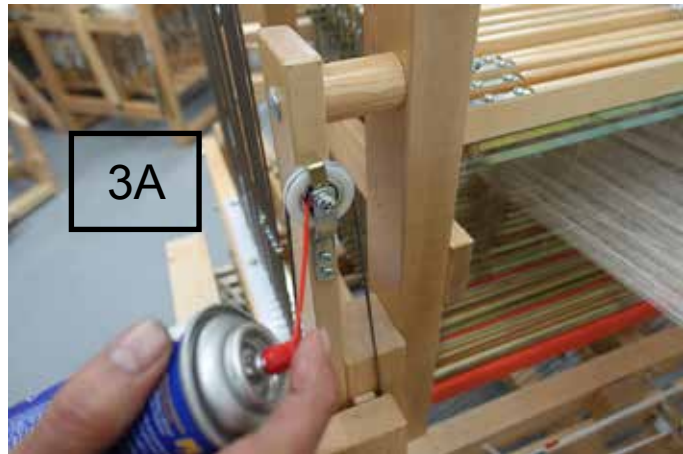
3- Spray into the ball bearing pulleys.
