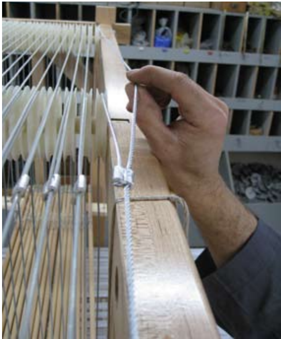
Make sure that the loop sleeves of the cables are parallel to the wood part of the shaft frame to avoid any damage on them.
